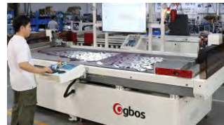
30度倾斜设计的铸造平台, X、Y、Z轴、基座均采用铸造一体成型工艺 30-degree inclined design casting platform X, Y, Z axes and base are cast in one piece.
