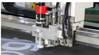
一体化刀座设计 (集合切割与冲孔) Integrated tool holder design (cutting and punching in one unit)
