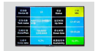
OEE看板, 实时查看设备运行状态、产能 OEE Kanban, real-time view of equipment operating status, capacity
