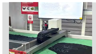
在线排版系统 边排版边切割, 极大提高效率 Projected real-time nesting or ITS3 online system Cutting while laying out the layout greatly improves efficiency
