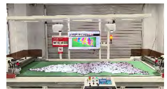
ITS3排版系统(选配) 半幅/全幅皮料、山羊皮等材料智能排版与切割 ITS3 Typesetting System (Optional) Intelligent Nesting and Cutting of Half/Full Width Leather, Goatskin, and Other Materials
